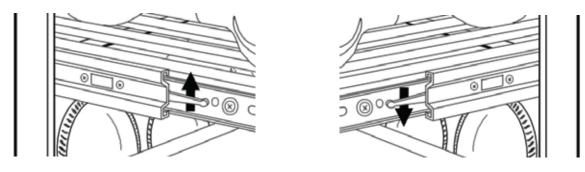
The shelves are removable to help with cleaning and maintenance. To remove a shelf, pull it out as far as you can. There are levers on each side of the shelf near the rollers. Lift the lever on the left hand side up and push down on the lever on the right hand side to remove the shelf from the tracks.
