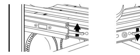
The shelves are removable to help with cleaning and maintenance. To remove a shelf, pull it out as far as you can. There are levers on each side of the shelf near the rollers. Left the lever on the left hand side and push down the lever on the right hand side to remove the shelf from the tracks.
